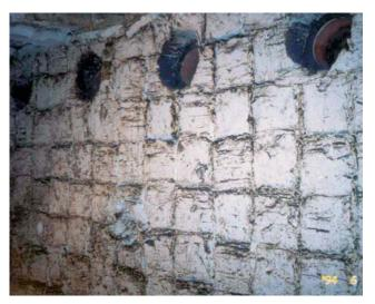
The existing lining in this batch forge furnace consisted of refractory ceramic fiber high temperature insulation modules on the sidewalls and endwall, with an IFB/bonded module roof. Due to the harsh operating conditions in this furnace, the sidewall modules had deteriorated, the bonded modules on the roof had suffered from spallation, and the underlying IFB had degraded significantly.
