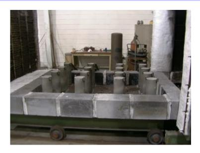
Refractory ceramic fiber high temperature insulation enables implementation of low mass designs in furnace car-bottoms, thereby offering significant fuel savings. The low heat loss and heat storage properties of Foamfrax High Temperature Insulation make it an ideal material in this application. Due to the support piers on these furnace cars, installation of either refractory ceramic fiber blanket or insulation modules can require extensive field cutting during installation.
