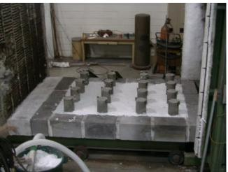
Foamfrax High Temperature Insulation is a gunnable, monolithic, thermally insulating material, that contains Fiberfrax refractory ceramic fiber as a major constituent.
