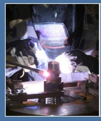
Our welders are AWS certified to ASME's Boiler & Pressure Vessel Code, Section IX -B31.1 and B31.3
